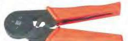
Capacity : 0.5mm<sup>2</sup> to 6mm<sup>2</sup>
